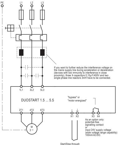
Start/Stop through contact or switching transistor optional control voltage 10 ... 42V DC (s. Commissioning Instructions)
